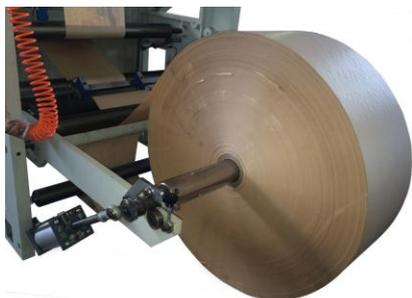
**Pneumatic paper reel lifting device**
